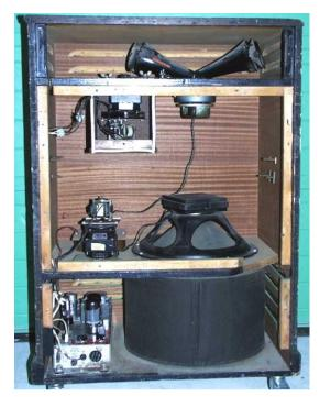
Fig. 1: The back side of a Leslie Model 147 speaker.
